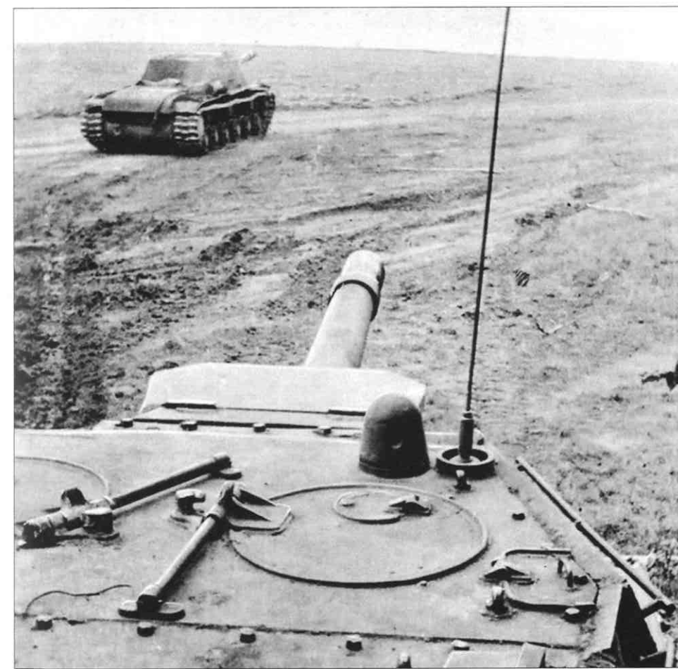
LEFT: ISU-152 Model 1944 SP guns on the move. The ISU-152, armed with a 152mm (5.9in) ML-20S with 20 rounds of HE and APHE ammunition, had a crew of five. The big gun fired a 43.4kg (96lb) shell to a maximum range of about 10,000m (10,935yd) and was more than capable of destroying the largest German tanks, as well as providing close support to infantry assaults against German fortifications and fixed positions.
