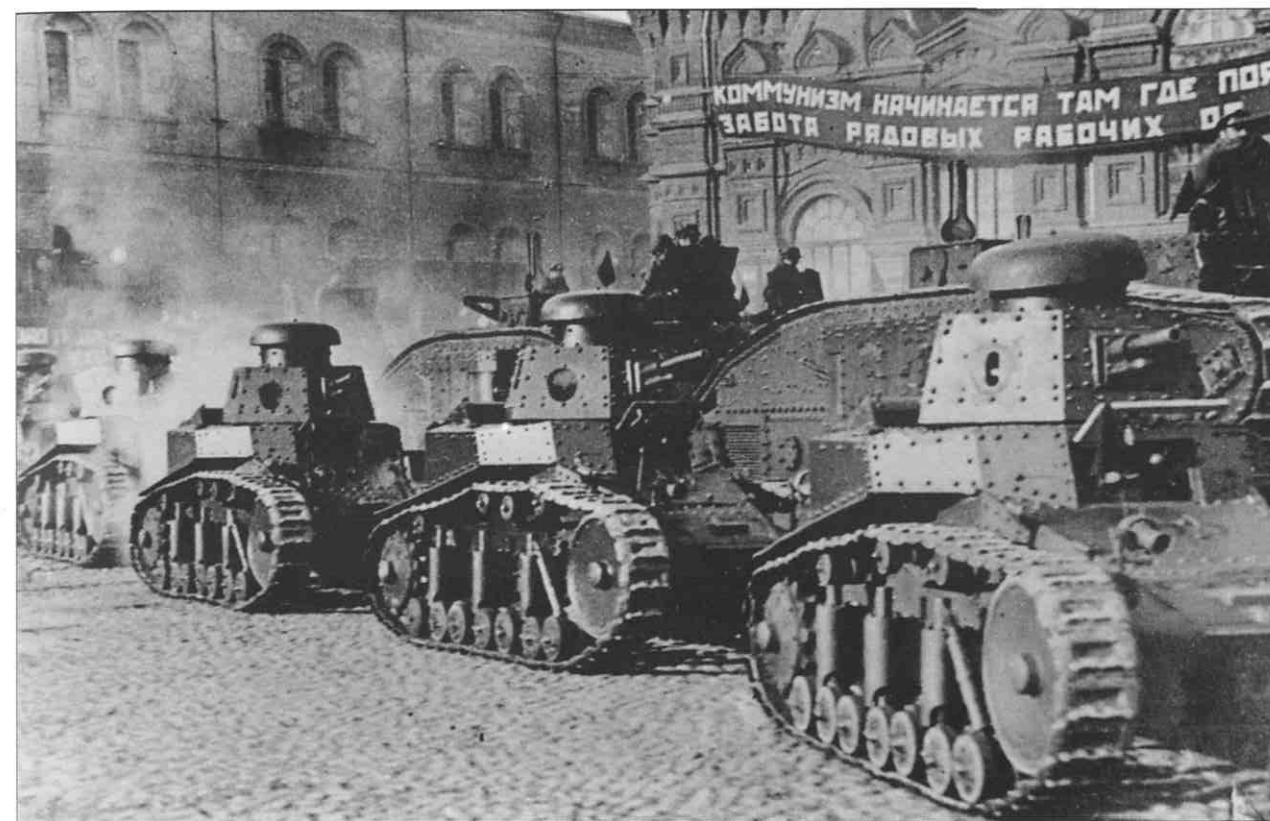
ABOVE: Amidst a cloud of exhaust fumes T-18 (also known as MS-1 Maliy Soprovozhdeniya-Pierviy : First Small Support Vehicle) light tanks move through Red Square during a May Day Parade. Production of this vehicle was plagued with technical problems, but between 1928 and 1931 some 960 T-18s were built. This was an altogether incredible achievement considering that this total was churned out even though production was halted to rectify serious design flaws, including adding a turret bustle and a more powerful engine.
