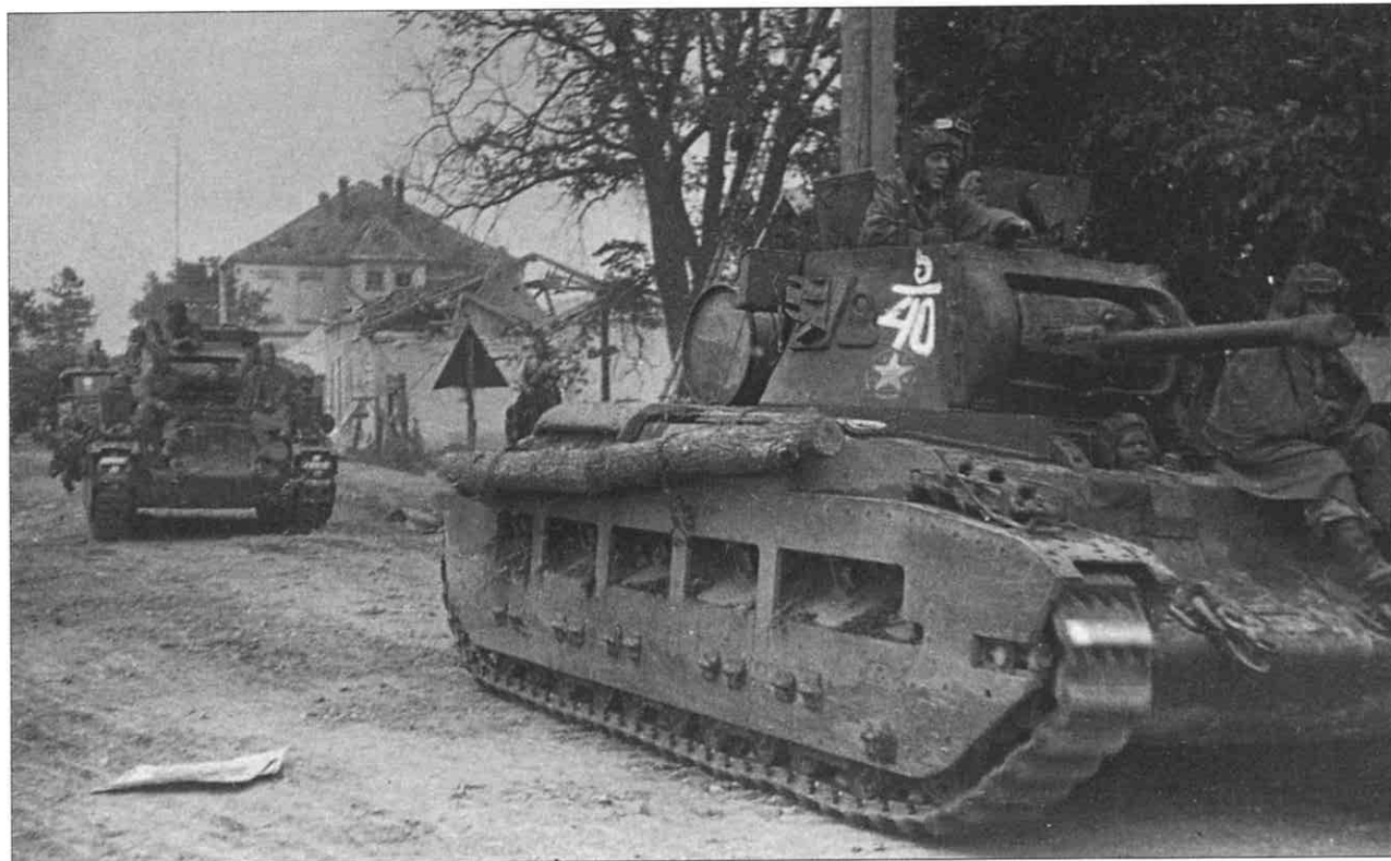
ABOVE: A Matilda II tank in the Ukraine in 1944, with a small tree trunk as an unditching beam and a fuel drum tied to the hull.
