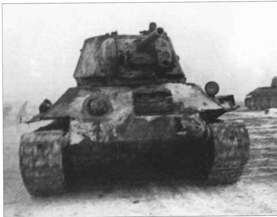
RIGHT: A T-34/76C Model 1943 named 'Leningradyets' of the 30th Guards Tank Brigade advances into Krasnoye Selo in January 1944. It had spudded tracks, single horn periscope, cast turret, twin driver's periscopes and an armoured shield on the hull machine gun, welded nose and claw tow-hooks on the glacis.
