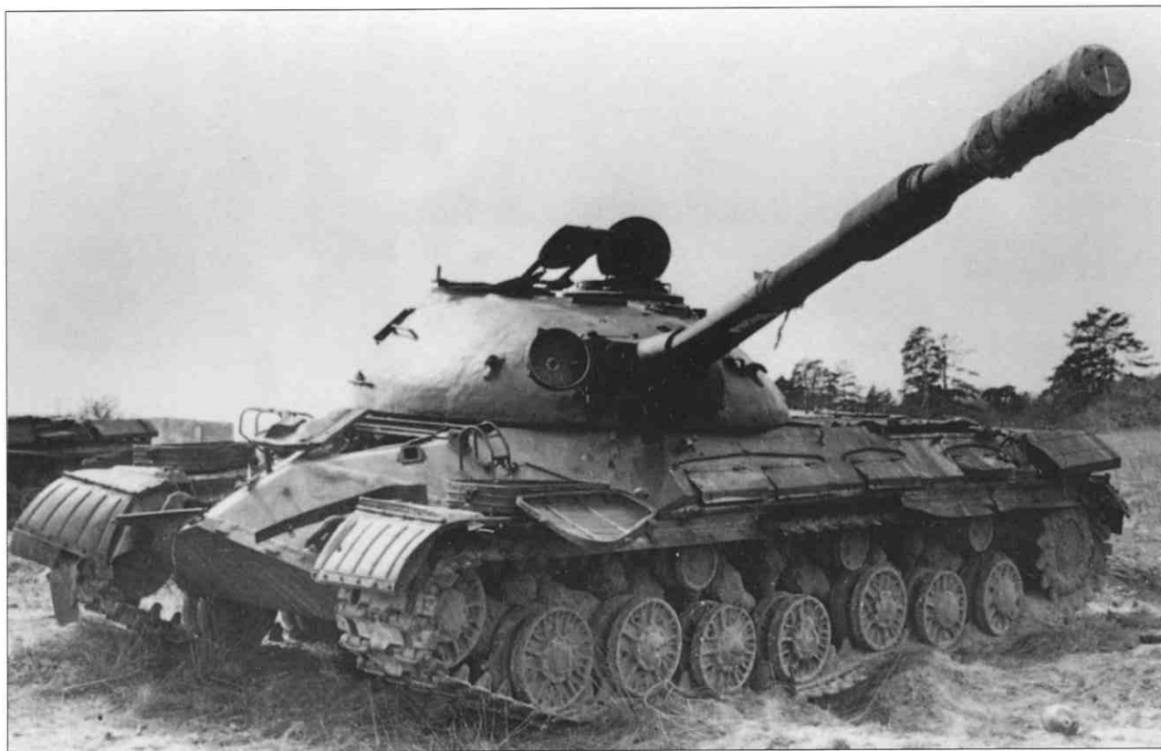
ABOVE: A battered T-10M heavy tank, with its distinctive 122mm (4.8in) gun with multi-baffle muzzle brake. It was the standard heavy tank of Soviet Ground forces during the 1950s and 1960s and was exported to Warsaw Pact allies and friendly nations. According to US estimates, the total post-war production of heavy tanks was about 9000 vehicles; about 1000 were IS-3M and IS-4, and the remainder were T-10 and T-10M.
