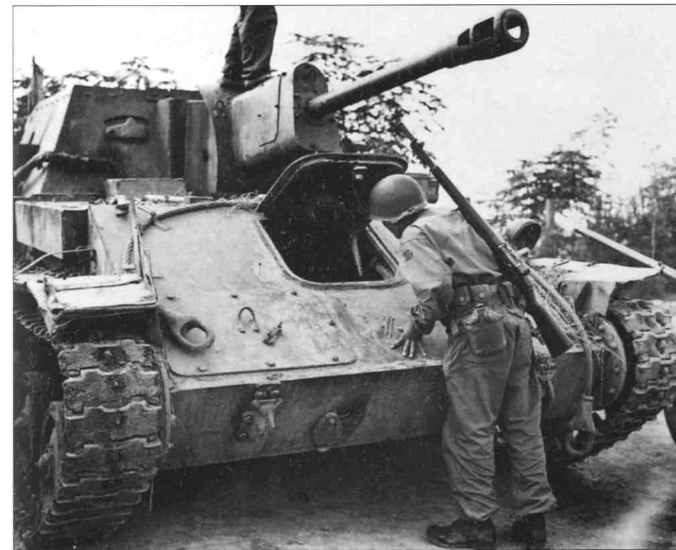
LEFT: Although despised by its crews, the SU-76M was an effective weapon which used the T-70's chassis. The vehicle was built in large numbers by the Soviets, and after the war continued to serve with a number of client states. In this photograph a Republic of Korea soldier inspects a captured SU-76M near Hayang in 1950, during the Korean War.
