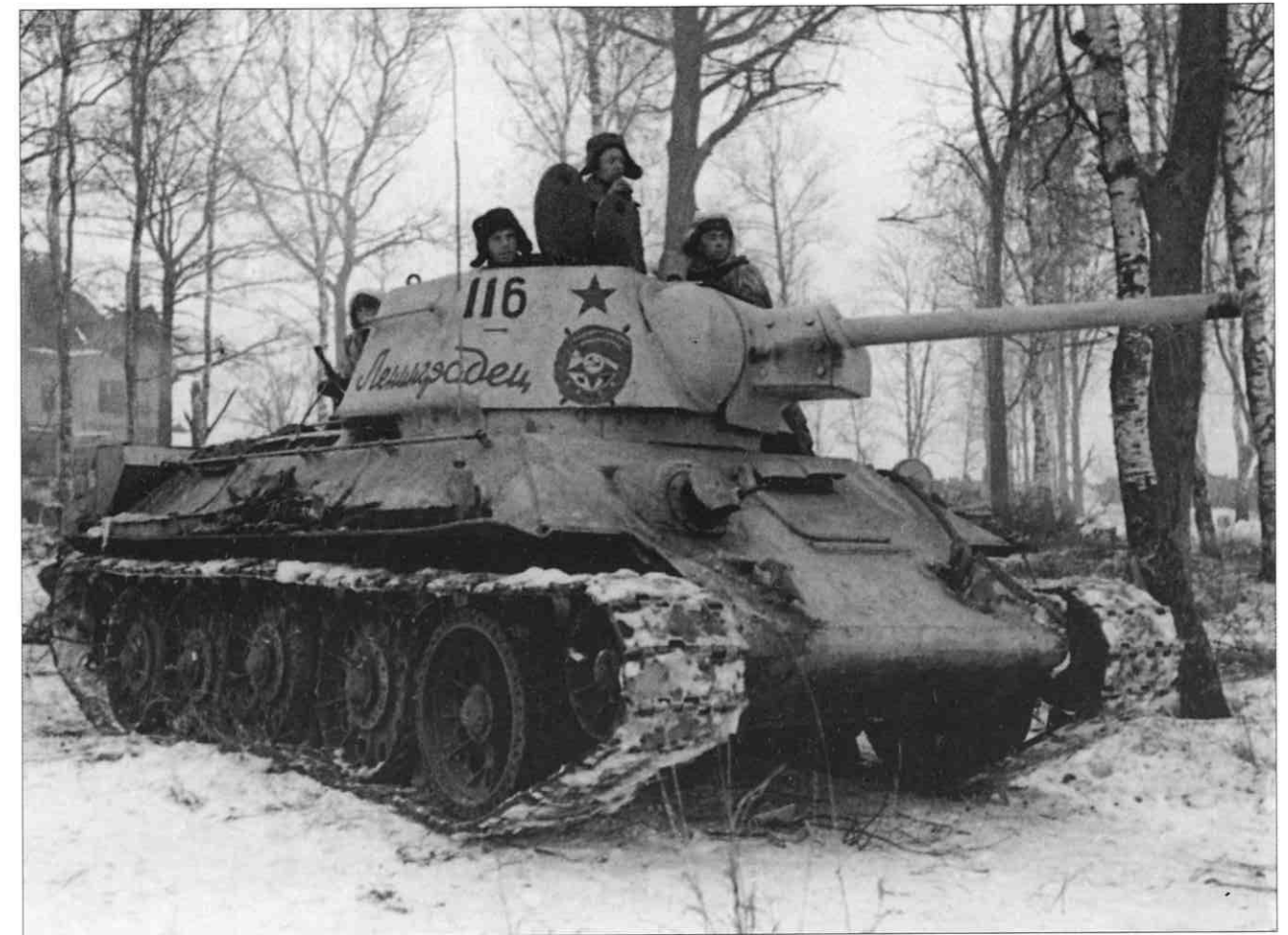
ABOVE: A T-34/76D tank advances across ground frozen solid in a hard frost in 1943. The big road wheels of the American-designed Christie suspension were less likely to jam up with mud and dirt when compared to the German tanks that had small road wheels and return rollers above them for the track. The German suspension system also left the side of the hull vulnerable to hits by antitank weapons.
