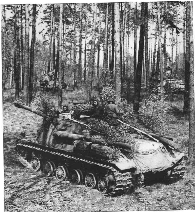
BELOW: Tyazholy Tank IS Heavy Tank 'Iosef Stalin' IS-2 tanks of the 1st Ukrainian Front camouflaged in a concentration area in woods near Berlin in April 1945. The IS-2 was armed with a 122mm (4.8in) M1943 gun with 28 rounds as well as a 12.7mm (0.5in) AA gun and three 7.62mm (0.303in) machine guns. The IS-2 was the most powerfully armed tank in World War II and its improved fire-control meant that it could fight German Tigers and Panthers on more than equal terms.
