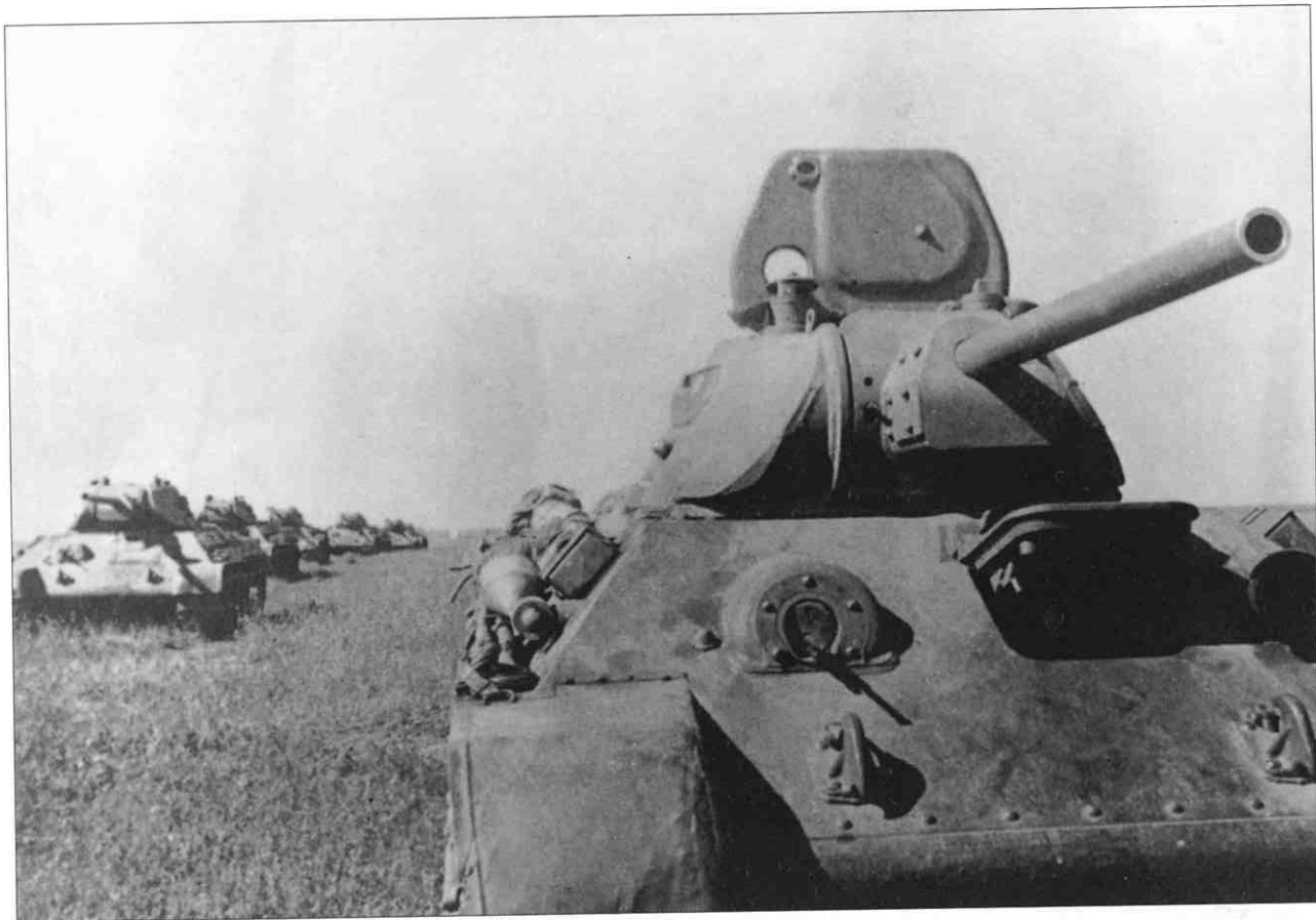
ABOVE: A tank formation, commanded by Major Baranov in a concentration area near the Crimea in October 1941. The smooth, well-angled glacis plate of the T-34/76B can be seen, with only a machine gun and the driver's hatch breaking the integrity of its armour protection.
