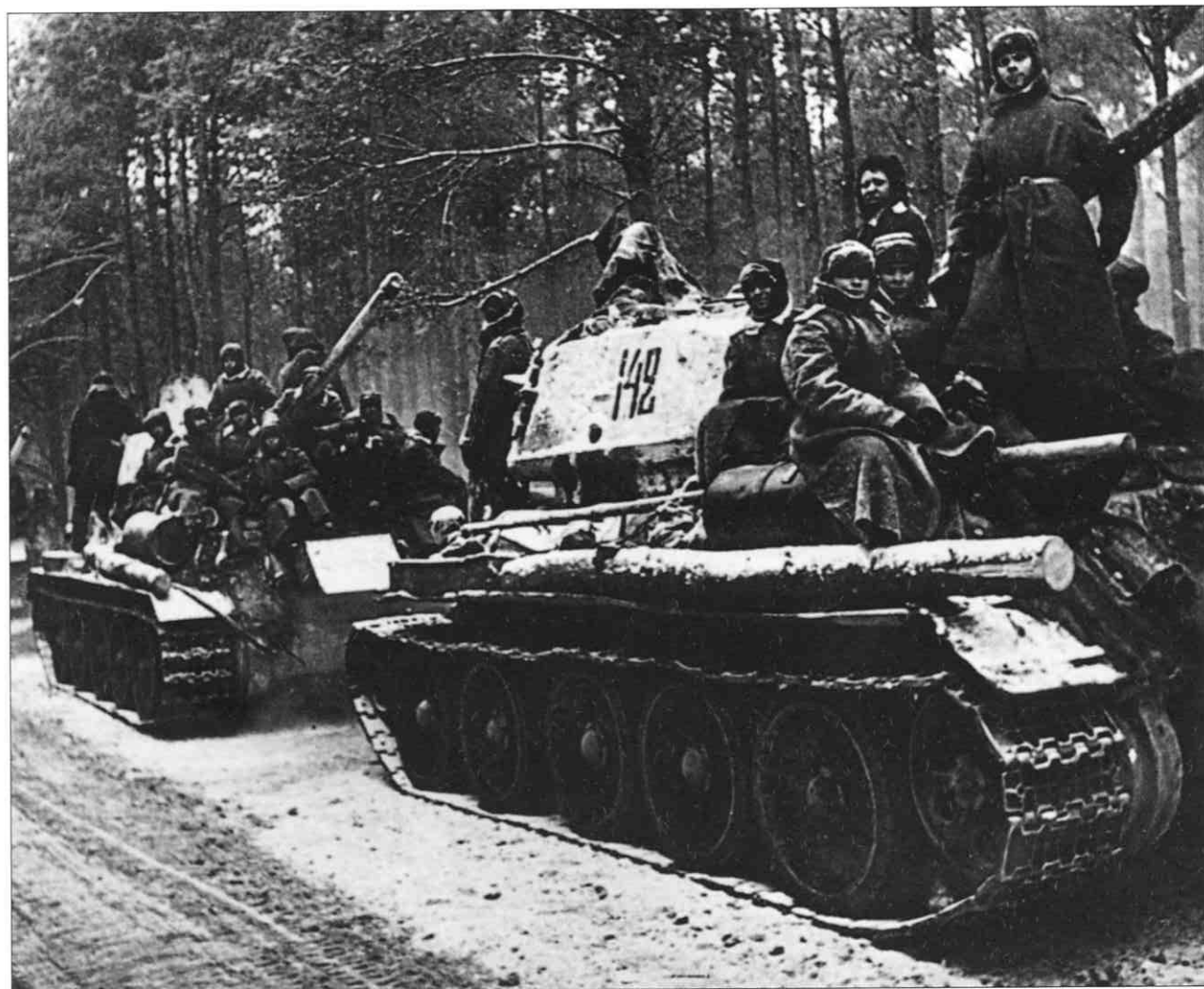
ABOVE: A column of T-34/85 with their turrets traversed to the rear in the winter of 1944. Early production models either lacked mushroom vents altogether or had one only and were designated T-34/85/1. The bigger turret allowed an extra crewman to be carried. The tank desants have collected on the louvres in order to enjoy the warm air which is wafting from the engines. An unditching beam has been lashed to the hull.
