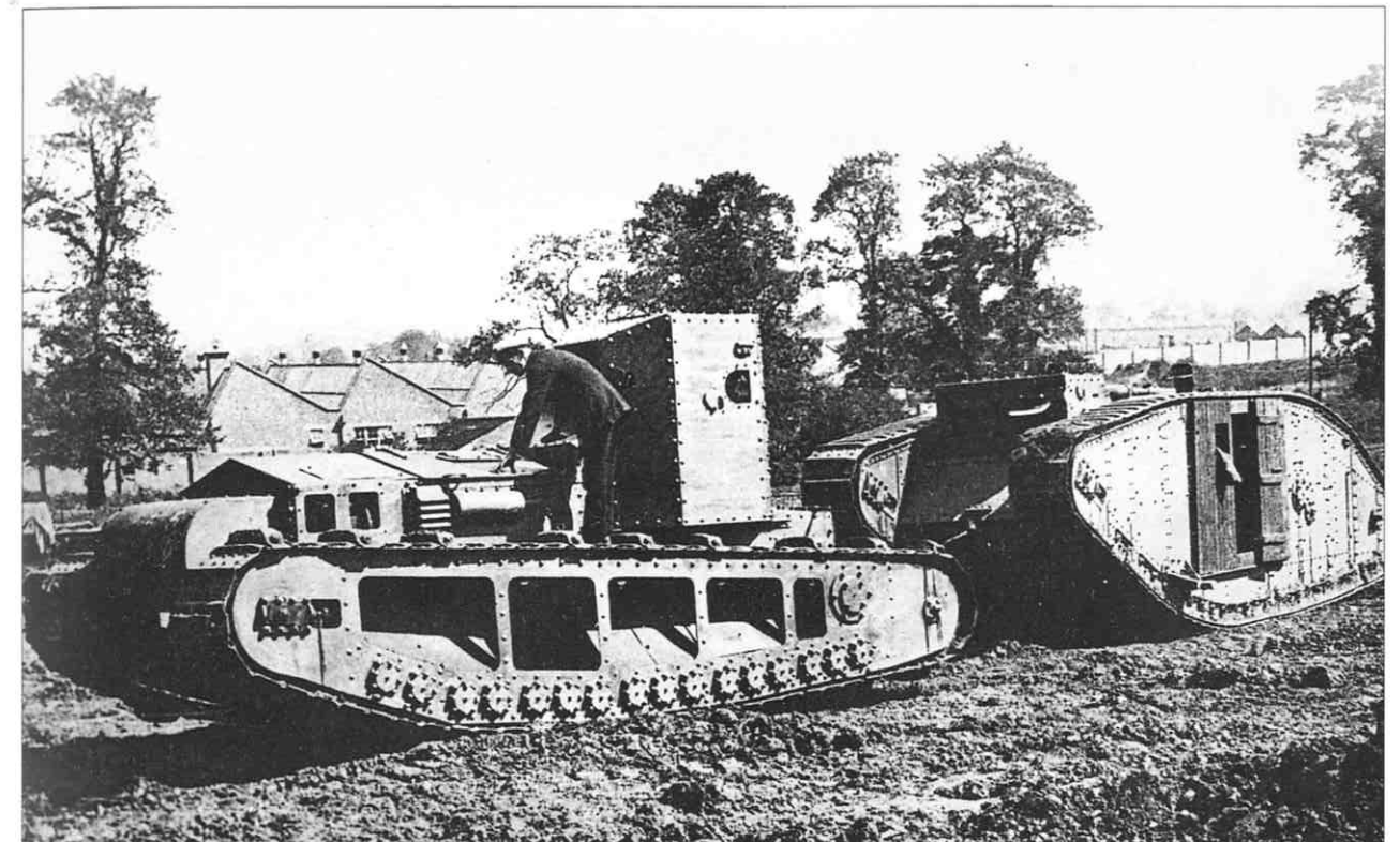
ABOVE: A Medium Tank Mk A, widely known by the British as the Whippet, and a Mk V that appears to have its gun sponson removed at a depot in France. Both types of tank were sent to Russia to assist in the fighting against the Reds, and examples of both were captured. The drive to industrialize the newly-formed USSR allowed Soviet engineers to retro-engineer captured tanks in the new factories that were being built, which encouraged the development of a Soviet tank industry.
