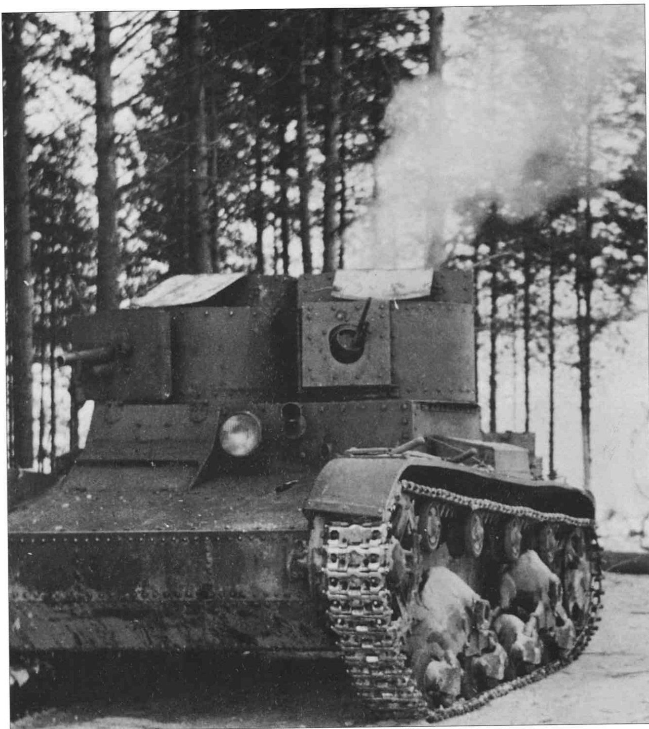
ABOVE: A T-26TU Model 1931 fitted with a Model 28 37mm (1.46in) gun in the left turret and a DT 7.62mm (0.3in) machine gun in the right. It carried 180 rounds of main armament ammunition on board, had a crew of three, and was usually assigned to platoon and company commanders.
