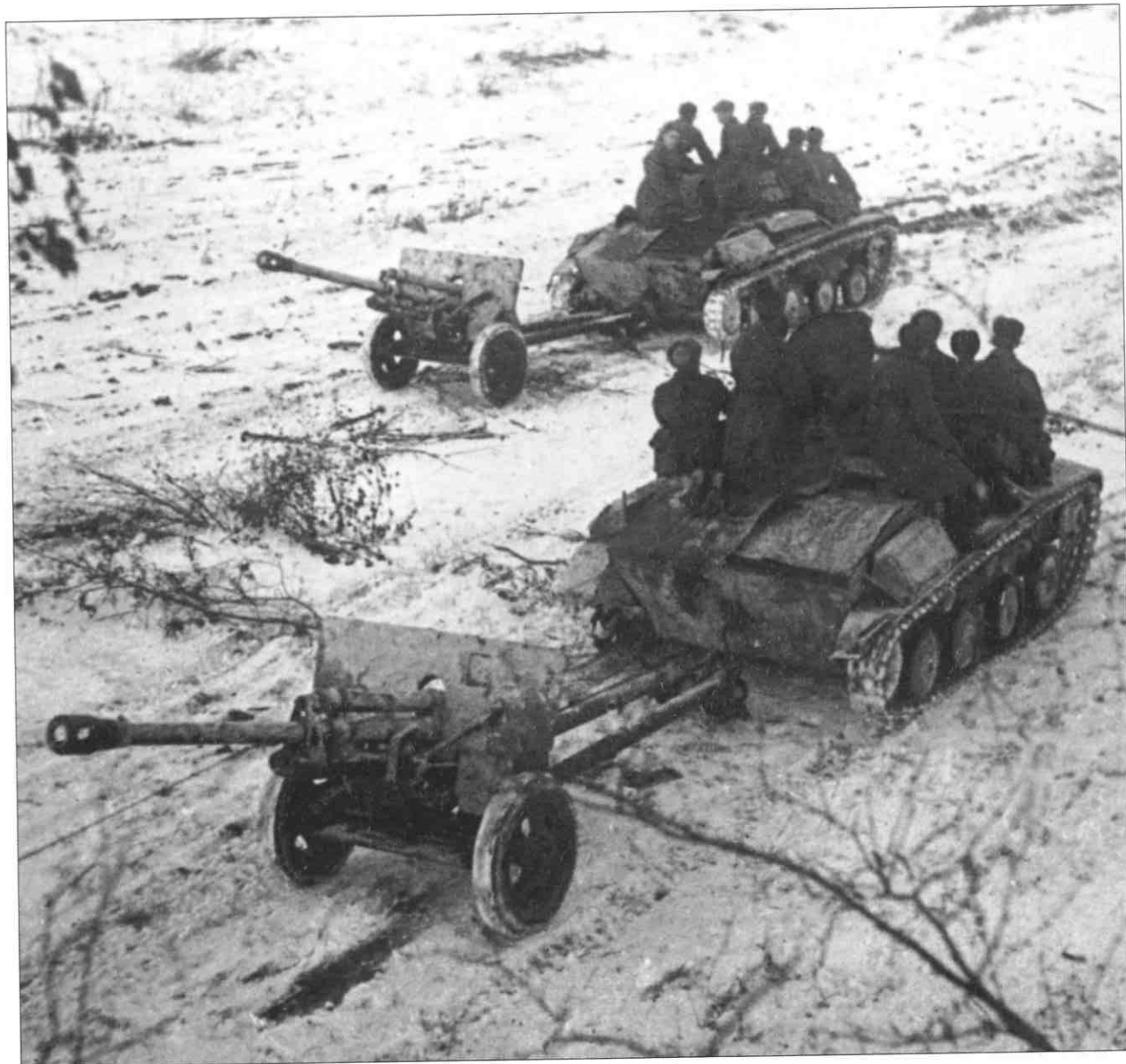
BELOW: A pair of T-70s are used as gun tractors by the crews of two M1942 ZIS-3 76.2mm (3in) antitank guns to move their weapons up to the front across the frozen ground. This photograph was taken near Leningrad in February 1943.
