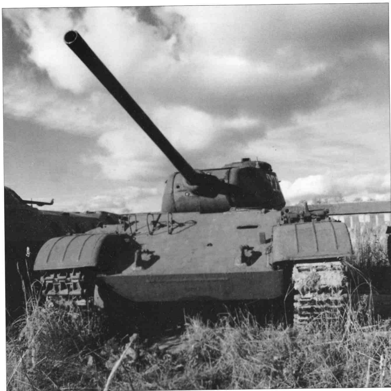
ABOVE: The T-44 developed by the Morozov design team retained the same turret as the T-34/85, as well as roadwheels, track and engine; however, the hull and engine layout was completely re-designed. New torsion bar suspension was added and armour protection for the turret front went up to 120mm (4.72in). A small number of T-44s saw action in the final months of World War II.
