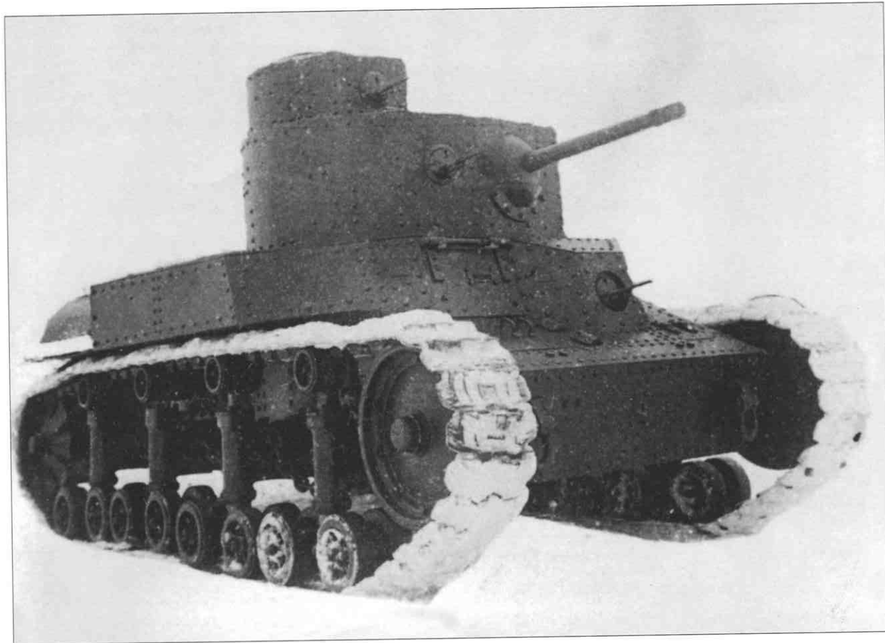
ABOVE: Developed around 1925, the T-12 had a 45mm (1.77in) gun with 100 rounds stowed on board. It was initially fitted with the distinctive 'tail' of the Renault FT-17 light tank. The T-12 was given a more powerful engine and also had a bigger crew than the FT-17. The commander had his own cupola with a machine gun. Although the 1930 budget had funds to develop 30 T-12s, the project was cancelled in favour of the T-24.
