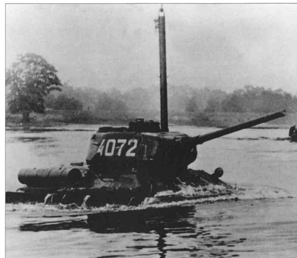
LEFT: A T-34/85 which is equipped with a snorkel submerged underwater during a river-crossing operation. In contrast to the standard postwar NATO practice in amphibious tank design, Soviet practice was to fit a snorkel which allowed in just enough air for the crew and the engine during short underwater crossings of obstacles such as rivers and creeks. However the air vent was not wide enough for the crew to escape through if the tank broke down under water – which could have fatal consequences for them.
